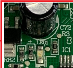
LED1: Drive failure indicator
