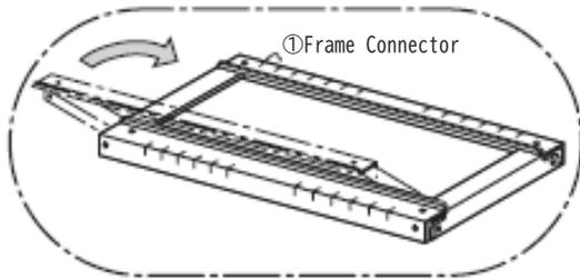
2. Raise up the ② Leg Connector set on the ① Frame Connector and fix it with the ⑧ Hex Bolts(+ M8-20)
