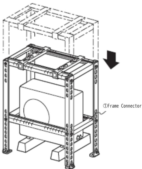
2. After preventing the air conditioner from tipping over, install the air conditioner in the upper section.
