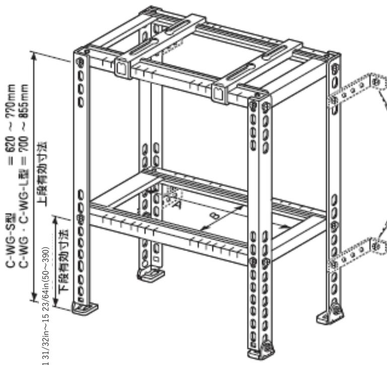
If the existing air conditioner is smaller than the effective inside dimensions, it can be used over the top.
