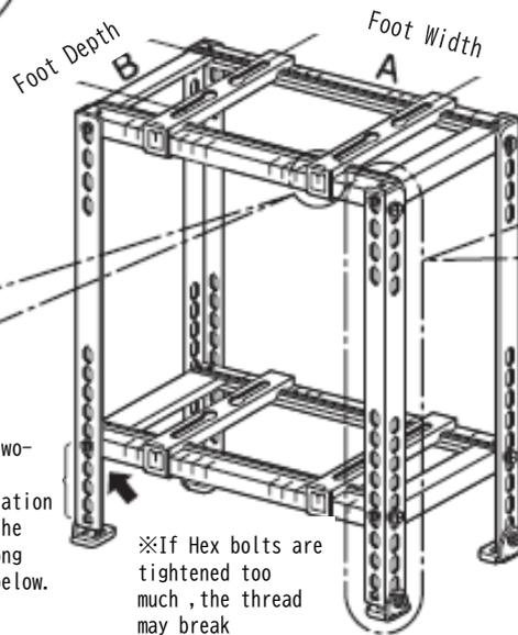
For a two-tiered installation, use the four long holes below.
