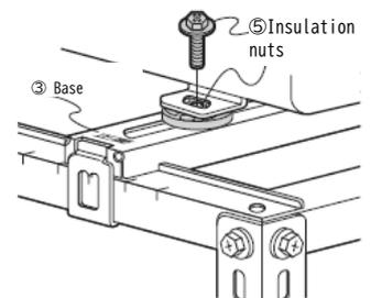
When used over an existing air conditioner (Back side for use as a two-tiered installation)
