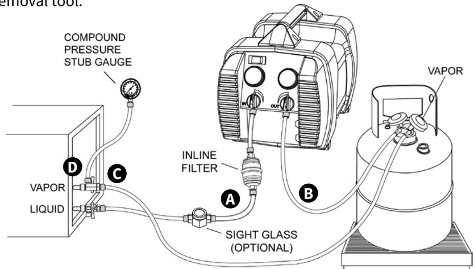
2. Close the Valve Core Removal Tool (VCRT) ball valves at both of the AC/R System Liquid and Vapor ports.
