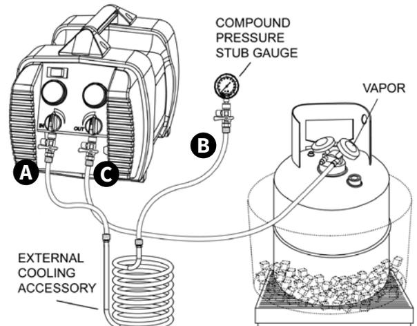
**WARNING:** After recovery is complete, the ECA and Hoses A, B and C will contain high pressure refrigerant.
