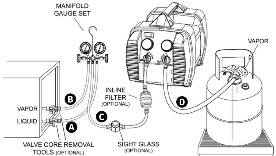
2. Close both valves on the Manifold Gauge Set.
