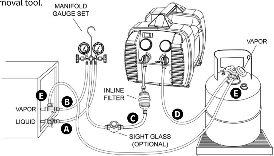
2. Close both valves on the Manifold Gauge Set. Open both valves on the G5Twin, open both valves on the Recovery Cylinder, and open the VCRT ball valves at the AC/R System access ports (if equipped).
