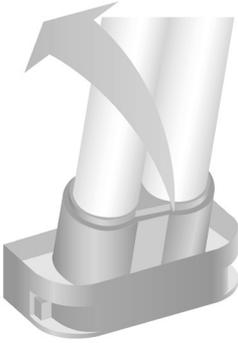
Fig. 4 UV lamp installation.
