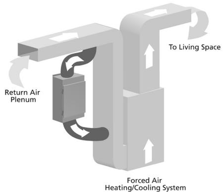
Fig. 3 Remote mount installation diagram.
