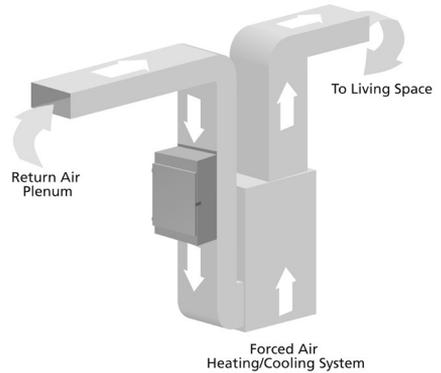
Fig. 2 Return air installation diagram.
