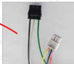
Polarized Molex Plugs Allowing for Simple Disconnect from Cabinet
