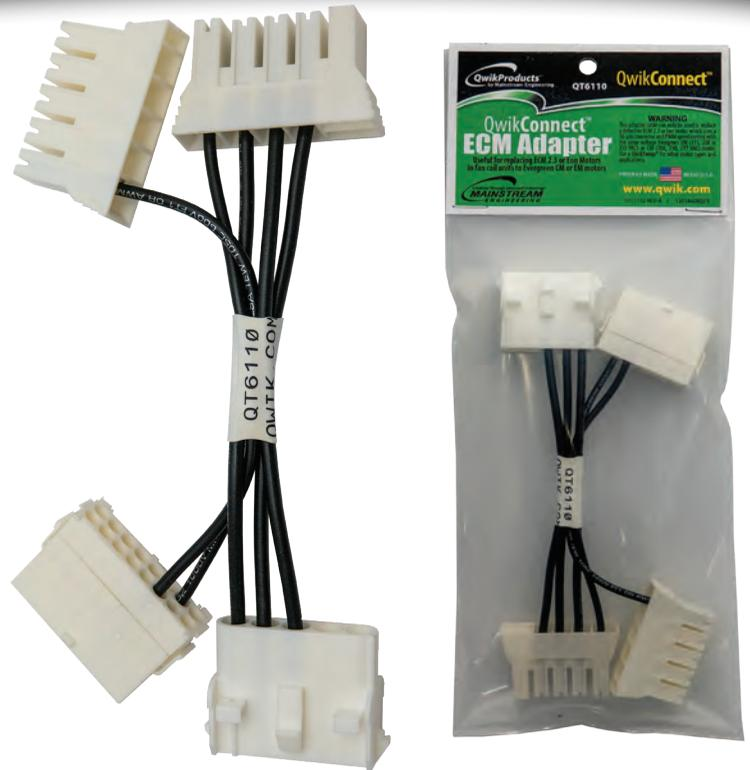
This adapter has two plugs on the one end to receive the plugs that were intended for an ECM 2.3 / Eon motor (J1 for Power, J2 for Communications). The signals from J1 and J2 are wired to the appropriate plugs for the Evergreen® Motor (P1 for Power, P2 for Communications).
