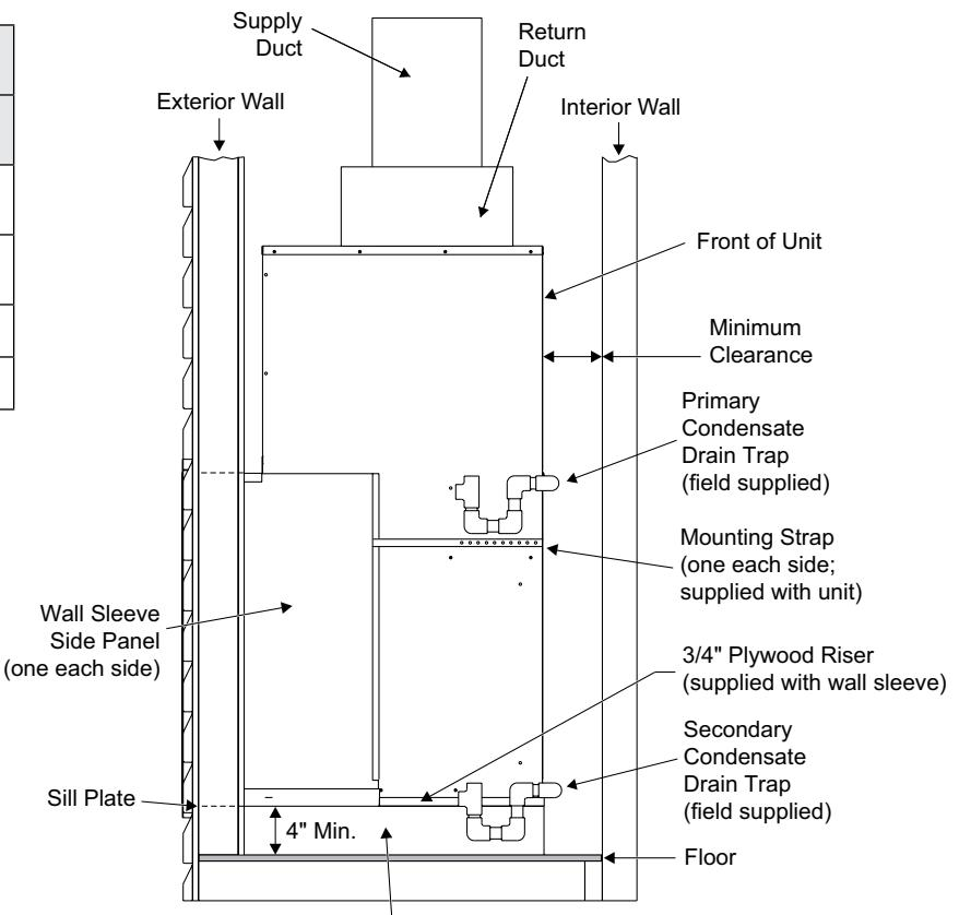
Platform (field supplied) - Unit must be supported by platform, which must be level with sill plate of opening in exterior wall.
