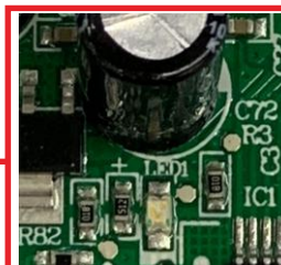
LED1: Drive failure indicator
