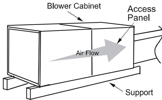
Figure 4 - Attic Installation
