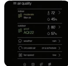
The **air quality screen\*** displays indoor air quality levels when a Daikin One home air monitor is connected. Outdoor air quality and weather will be displayed when connected to the internet and thermostat added in the mobile app under home location.
