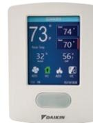
The Daikin *Adaptive Touch Controller* (ATC) is used to control FDMQ, FFQ & *SkyAir* indoor units with advanced and configurable control logic. The *ATC* comes in 4 different models with a built-in temperature sensor, humidity sensor, CO<sub>2</sub> sensor, and occupancy sensor.
